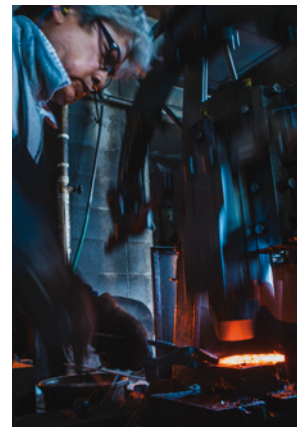
Below right: Tsukasa Hinoura is forging a billhook at Hinoura Hamono Koubou, Sanjo
